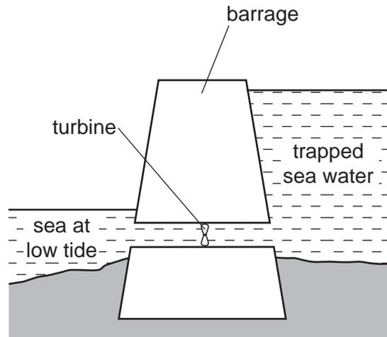
At low tide the water is allowed to flow back into the sea through a turbine.
